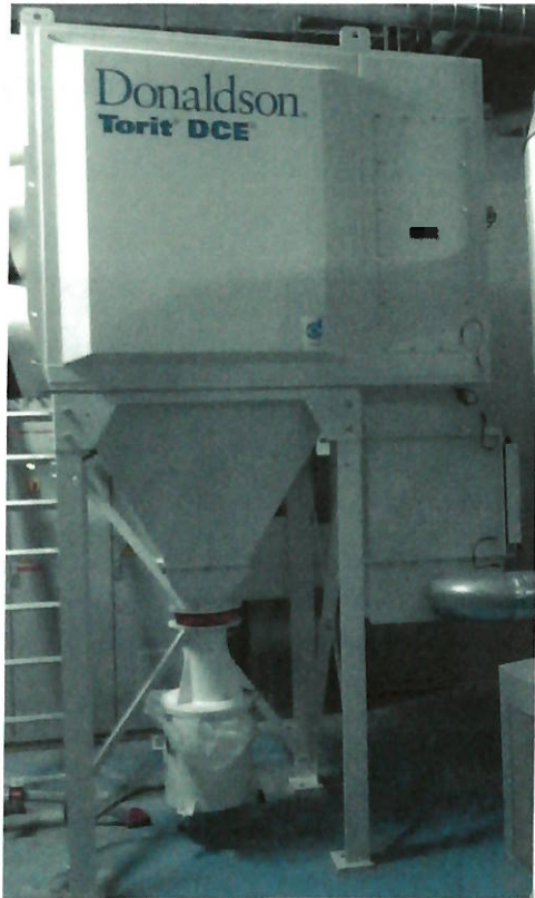
Figure 23. Dust Collecting Unit
